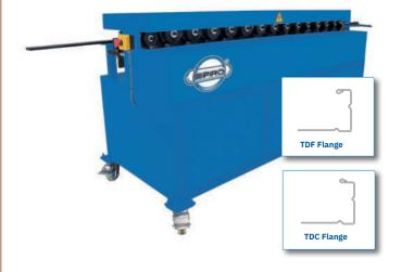
This 14 station Rollforming Machine makes a rigid TDC or TDF flange from hand fed blanks using material from the duct wall.
